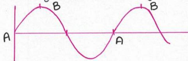
(ii) For a wave on the string, both the K.E. density and P.E. density is maximum near the mean position of the particle and it is minimum near the extreme position of the particle.
