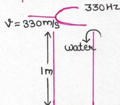
Ques.) An open organ pipe has a fundamental frequency 330Hz. The first overtone of a closed pipe has the same frequency as first overtone of this pipe. How long is each pipe. Take  $v = 330 \text{ m/s}$ .
