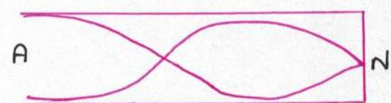
Ques.) A pitch pipe of length 1m is excited using a tuning fork of frequency 330Hz. Now water is gradually poured into the pipe. For what levels of water would you observe resonance?
